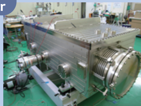
Dimensions : 900mm W x 2000mm L x 600mm H Tin sheets are used for sealing the rectangular flanges.
