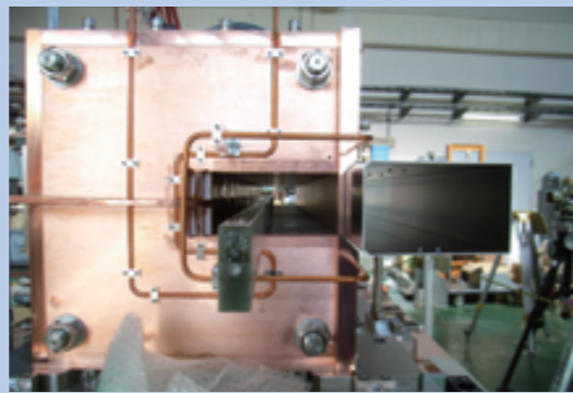
▲ Magnetic Field Measurement with beam pipe
