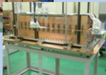
The laminating structure of non-directional silicon steel plates with 0.35mm thickness
